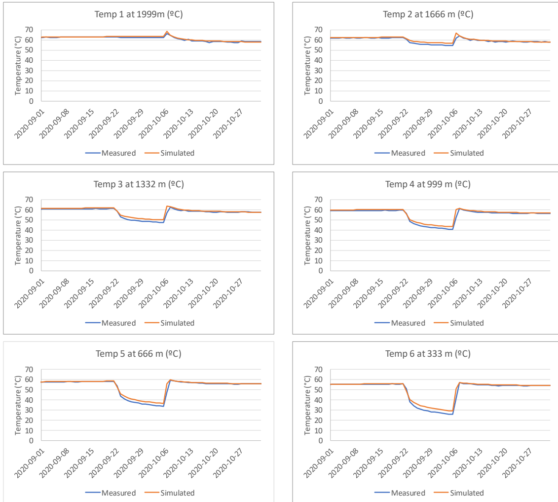
Figure 3: Measured and predicted temperature falloff in the outlet well thermocouple during the thermal recharge test
